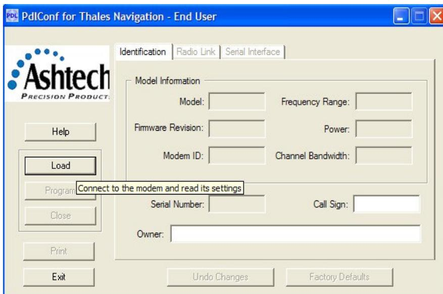
PDLCONF will read information from the radio and display it on the three tabs shown on this window.
