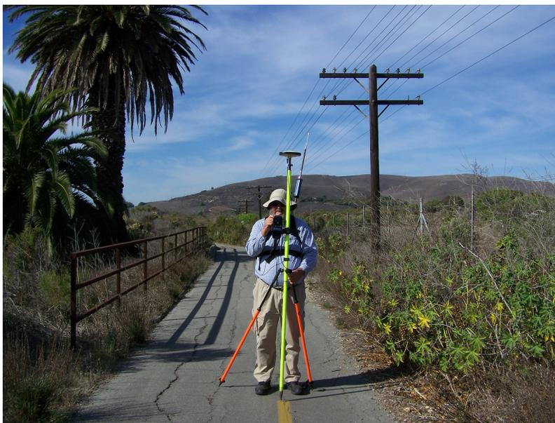
Some people have asked why the PDL rover radio was mounted on the SECO backpack that I typically use to mount the NAP100 antenna for Mobile Mapping work. The pole bracket for the rover radio was not available during testing. Contact your dealer about the pole bracket made by SECO.
