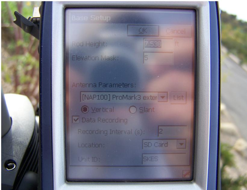
Data recording is not required for RTK work but the raw data file can be used in GNSS Solutions to compute even more accurate base station coordinates relative to the CORS or another ProMark3 set on a geodetic control point.
