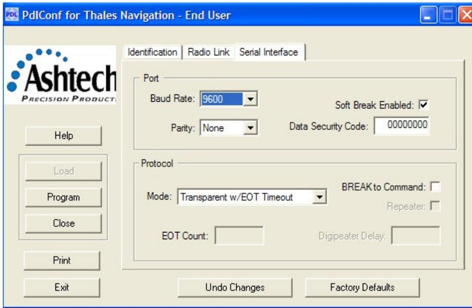
Click the Program button to send your changes to the PDL radio then click the Close and Exit buttons to disconnect from the radio and exit from PDLCONF.
