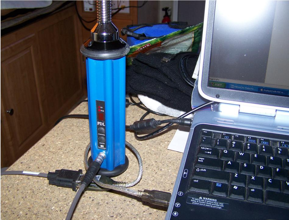
The rover PDL uses its own internal battery that is charged only while the rover radio is turned on and connected to the charger. While it is charging the LED display has a rotating line going around it. When the internal battery is fully charged **F** will appear on the LED display. This PDL rover radio is ready for a click on the Load button.
