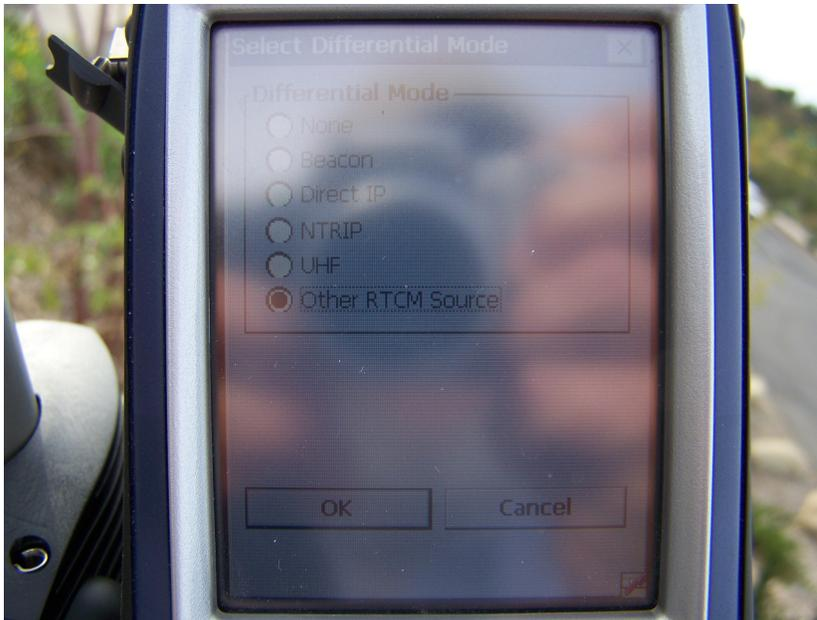
Open the DGPS Configuration menu from the ProMark3 desktop and choose Other RTCM Source. The base station will receive differential corrections from the SBAS. This configuration will set the base to send corrections using the settings appropriate for the PDL base radio as it was configured using PDLCONF.
