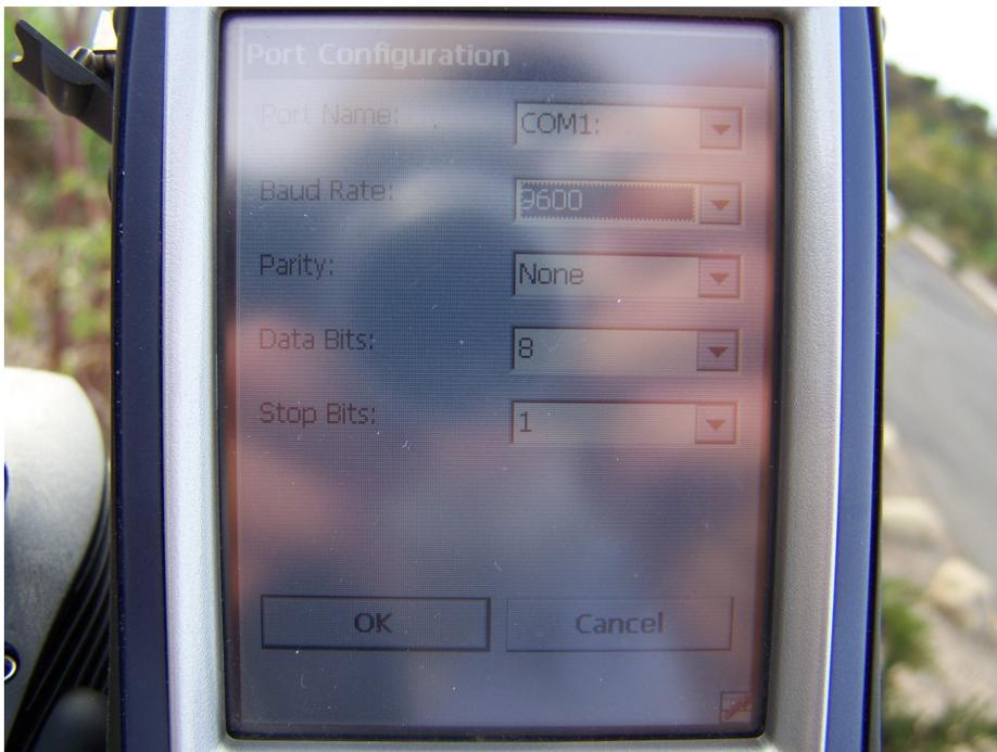
The PDL base radio on COM1 with a Baud Rate of 9600. Parity None, Data Bits 8, and Stop Bits 1 completes the settings for the connection to the PDL base radio. Tap the OK button to apply these settings. Tap the Connect button to make the connection to the PDL
