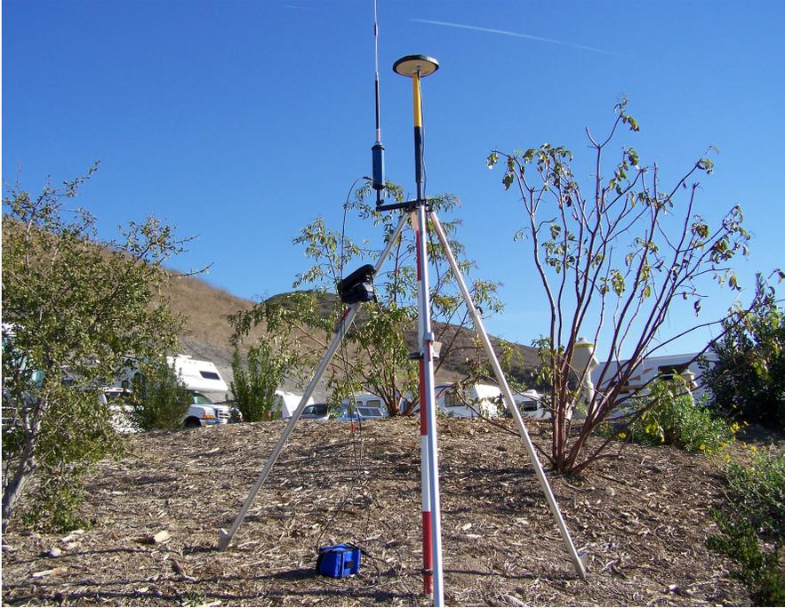
After the ProMark3 boots up check to make sure the clock sets properly. Wait for the GPS signal to set the clock.
