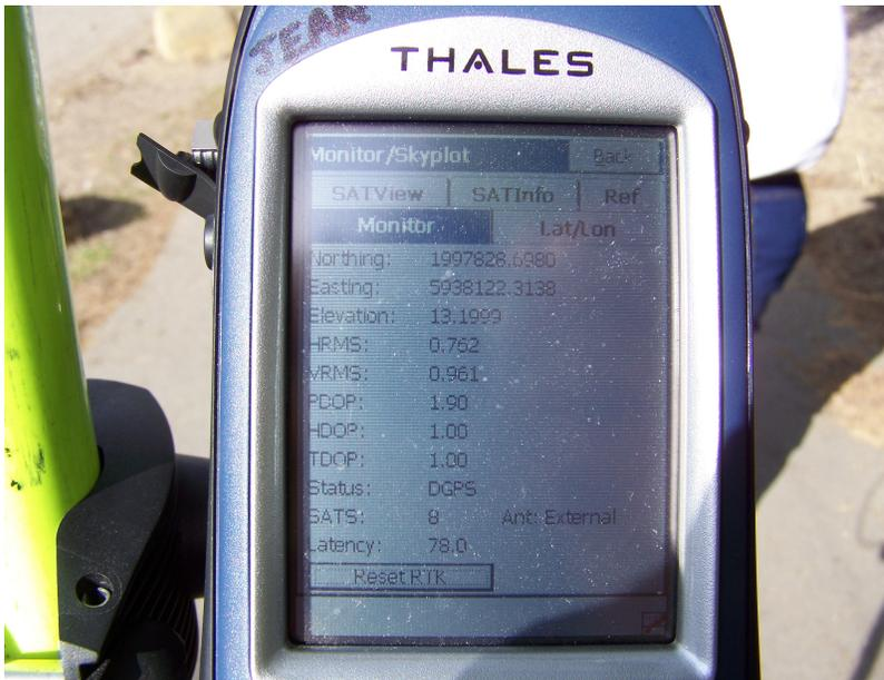
If the data link is lost the ProMark3 rover will default to a DGPS solution using the SBAS. The latency of 78.0 indicates that the radio data link is not working. Can this be explained by *The Guide to Wireless GPS Data Links*? Is the portable scanner picking up a signal from the base? Are the base and rover batteries providing adequate power?
