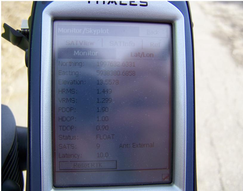
A latency of 10 is rather high. When the radio link is performing well the latency will typically be near 2.0
