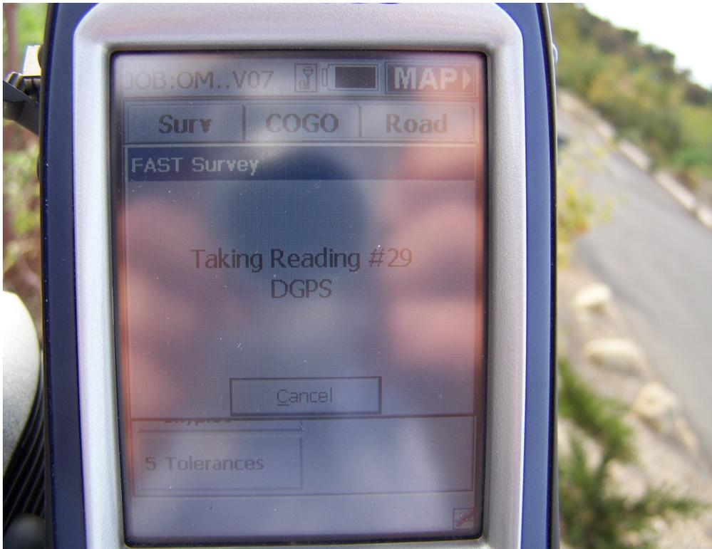
Thirty seconds passes quickly. The next screen shows the base station coordinates that will be used for the corrections. Localization, if desired, will be done at the rover.
