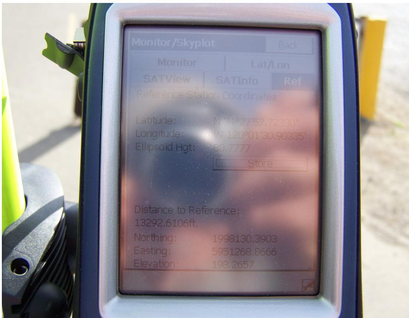
Check the Ref tab to see where the base station is located. This fixed solution 2.5 miles from the ProMark3 RTK base was good news. It was also a reasonable number. This indicates that the corrections being used are coming from the base station that was set up for this project. Tap the Store button to record the base station coordinates in the rover data file.
