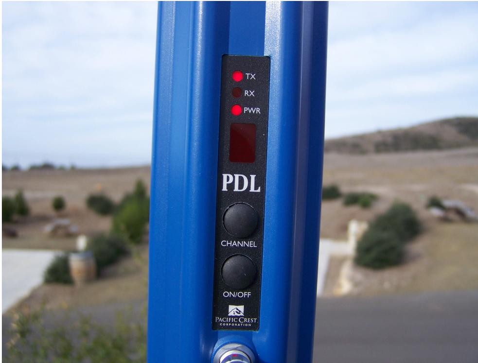
With the ProMark3 RTK base station set the PDL base radio begins blinking the TX light at a uniform interval. A RX light indicates competition for the selected frequency. A different channel must be selected if the RX light is on and the TX light is not blinking.
