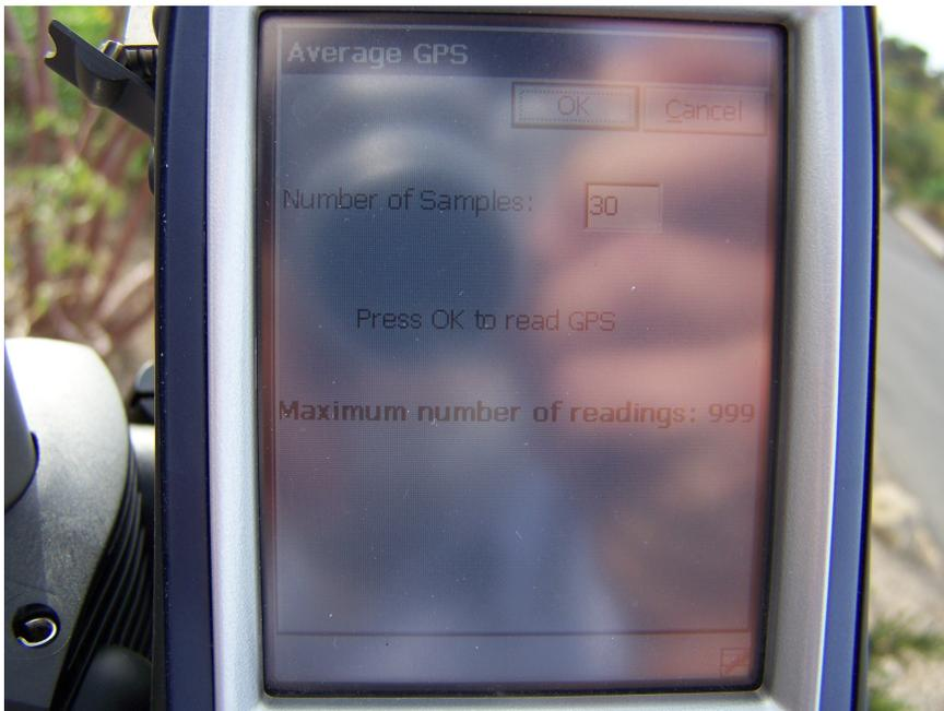
An average of 30 readings will help record a good base station position for the RTK work.
