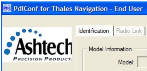
Click on the small square button with PDL in it at the top left corner of the PDLCONF window to bring up a software configuration window.
