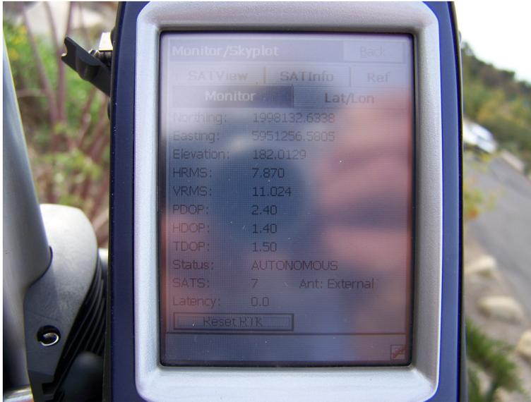
Before setting the base check to see what kind of position is being computed. Evaluate how good the position is. The autonomous position is not bad but waiting for a DGPS solution with the SBAS will improve the accuracy of the base station coordinates.
