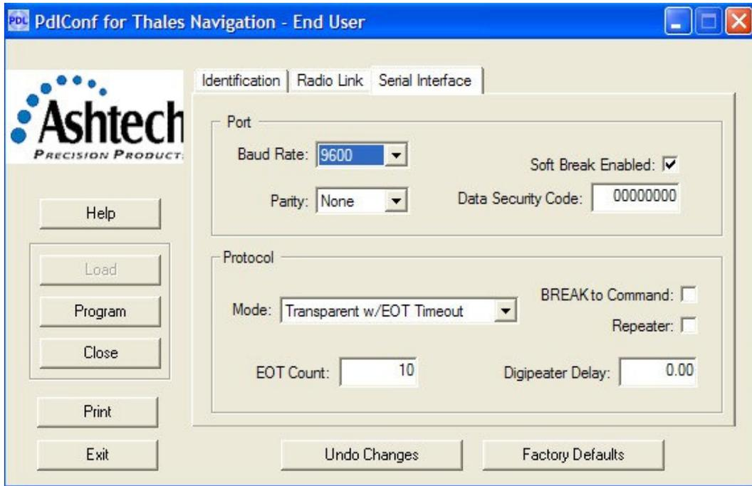
The serial interface relates to communication between the ProMark3 and the PDL. The settings illustrated were used during testing.
