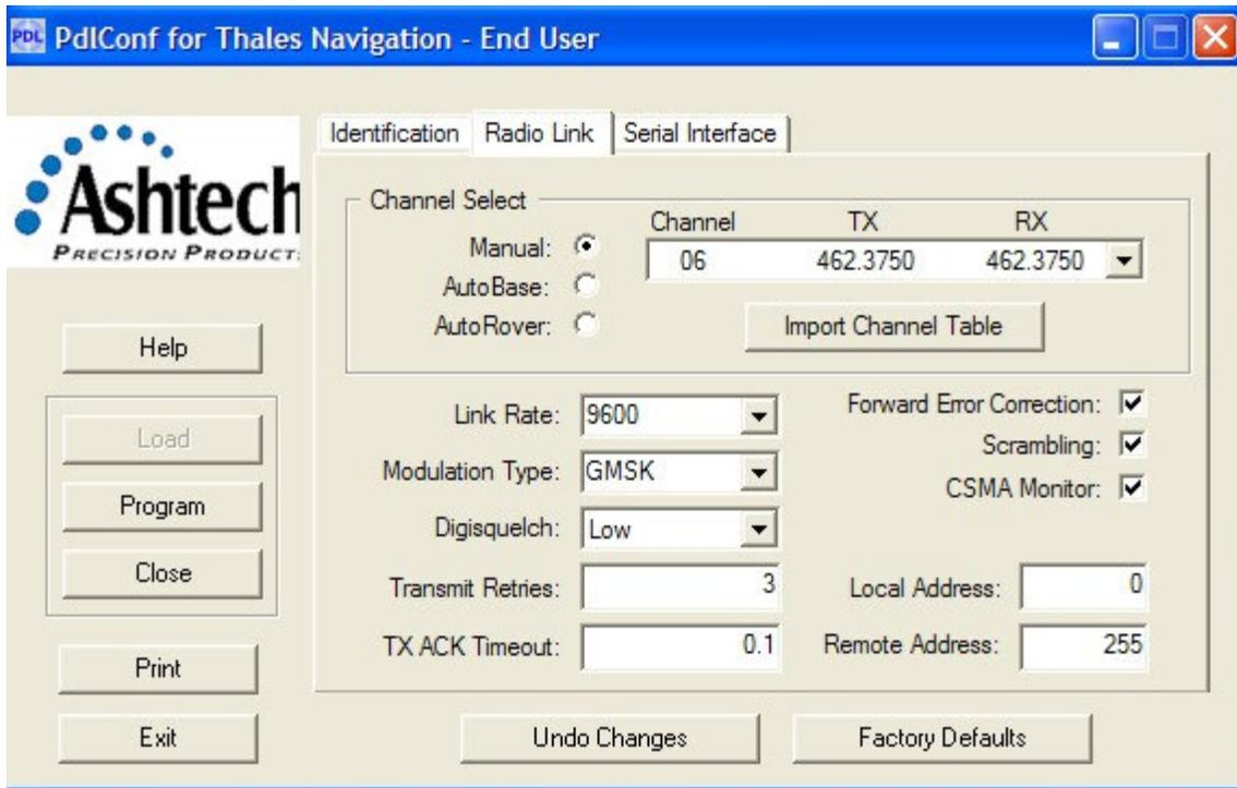
The Radio Link settings determine how the base and rover radios will work together. This is not the only possible way to configure the base radio. This illustrates how the radios were configured for testing the system.
