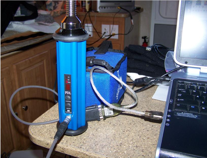
This PDL base radio, with antenna mounted and battery connected, is ready for the connection to the PDLCONF software through a USB to Serial adapter cable.
