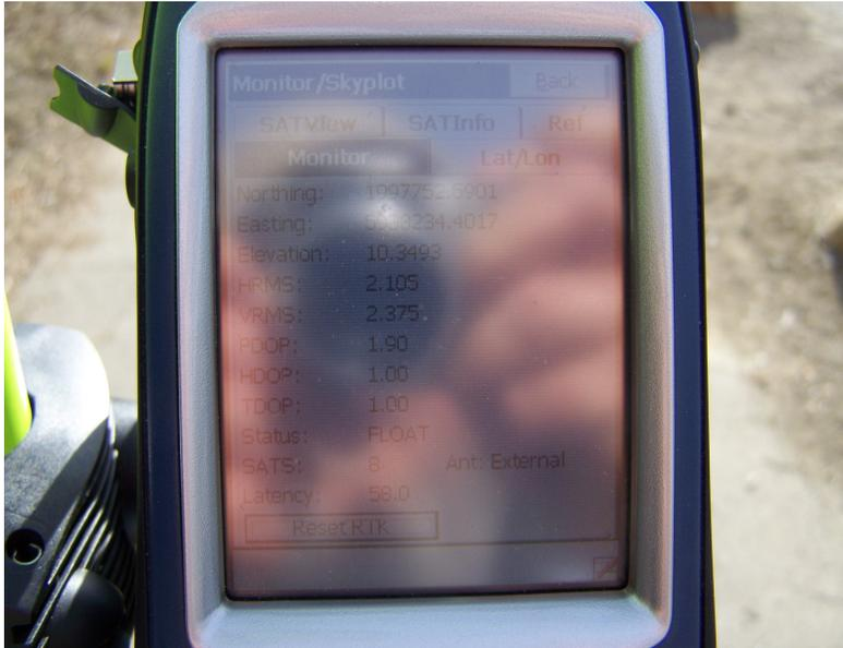
This Float solution with a Latency of 58.0 indicates that the data link has been lost. The HRMS and VRMS are accuracy estimates. The estimates do not guarantee accuracy nor do they measure the potential for error.
